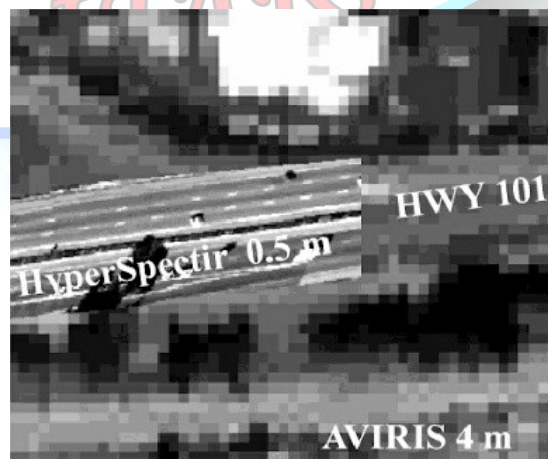
Figure 3: Visual different between hyperspectir (0.5 m) and AVIRIS (4 m) data emphasizing expected limitations due the spatial resolution configurations.
