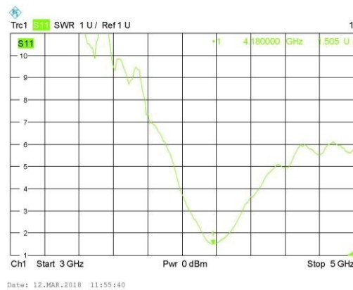
Figure 8 : Ref. MPA VSWR measurement result chart results.
