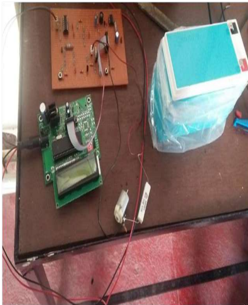
Fig. 4. Hardware Prototype of the buck converter
