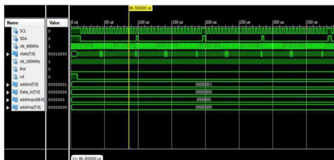
Fig. 10 Master I 2 C bus protocol simulation result
