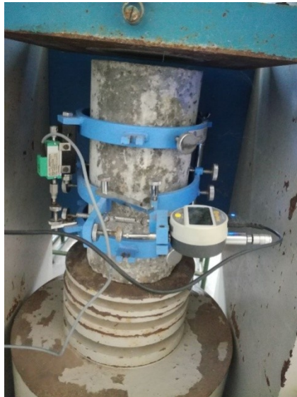
Fig 6: Young's modulus test setup
