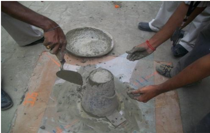
Fig 3.1 slump flow test.
