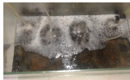
Fig.6 Working of Lab scale MBBR using Conventional Carrier (AnoxKaldnes™K1)
