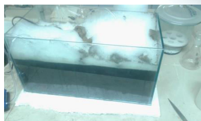
Fig.5 Working of Lab scale MBBR using Eco-friendly Carrier
