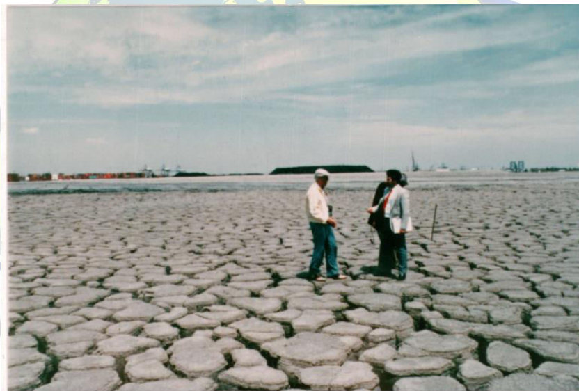
Fig. 2 Uneven desiccation cracking
