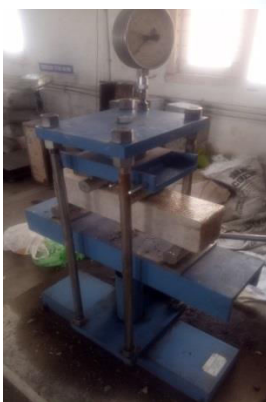
Fig 5.2 Test Set Up for Flexural Strength
