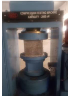
Fig 5.1 Test Set up for Compressive Strength Test
