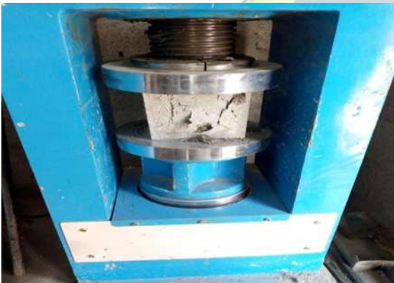
Fig 11 COMPRESSION TEST FOR CUBE
