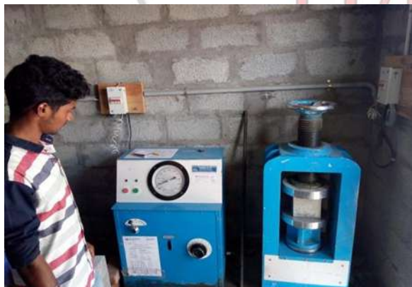
Fig 12 COMPRESSION TEST
