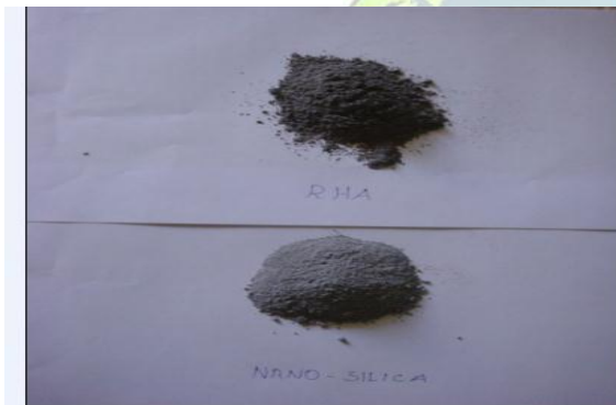
Fig.3 RICE HUSK ASH (TOP) NANOSILICA (BOTTOM).
