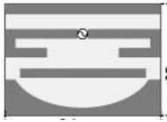
Figure 5 : Layout of the proposed antenna element.
