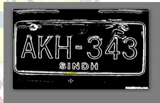
Fig. 3 Edges are detected by canny edge detector.
