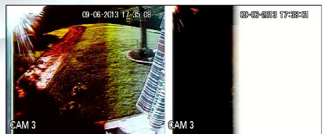
Figure 1 Sun Induced Burn Out Problem on Security Cameras
