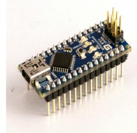
The Arduino Nano is a small, complete, and breadboard-friendly board based on the ATmega328 (Arduino Nano 3.0) or ATmega168 (Arduino Nano 2.x). It has more or less the same functionality of the Arduino Duemilanove, but in a different package. It lacks only a DC power jack, and works with a Mini-B USB cable instead of a standard one. The Nano was designed and is being produced by Gravitech.
