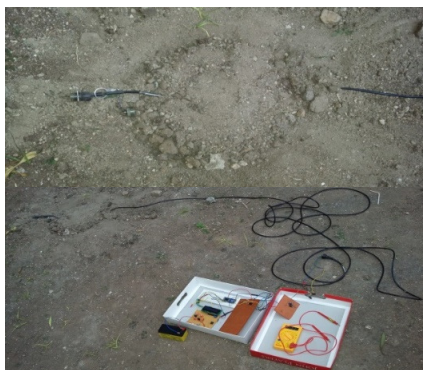
Fig 7 Hardware Setup while recording the values from Geophone and Moisture Sensors
