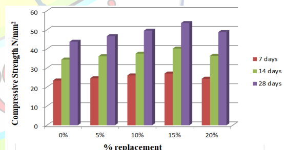
Fig 6.1 Avg. Compressive strength of geopolymer concrete with different % replacement
