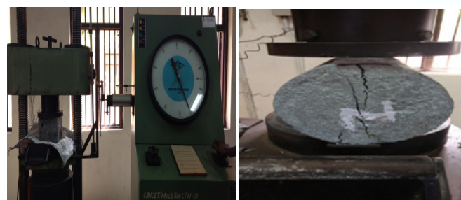
Fig. 3 Compression and Split Tensile strength test of specimen
