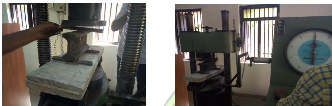
Fig. 3 Flexural test of specimen
