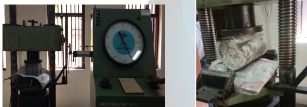
Fig. 4 Compression and Split Tensile strength test of specimen
