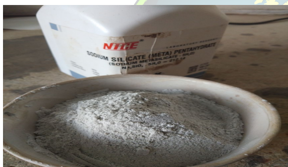
Fig. 1 Soil stabilizers are Marble dust and Sodium silicate
