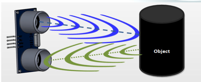
Fig.9.Working of ultrasonic sensor
