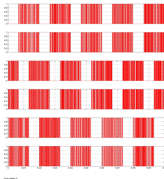
Fig.9. Pulses Given to the MOSFETS
