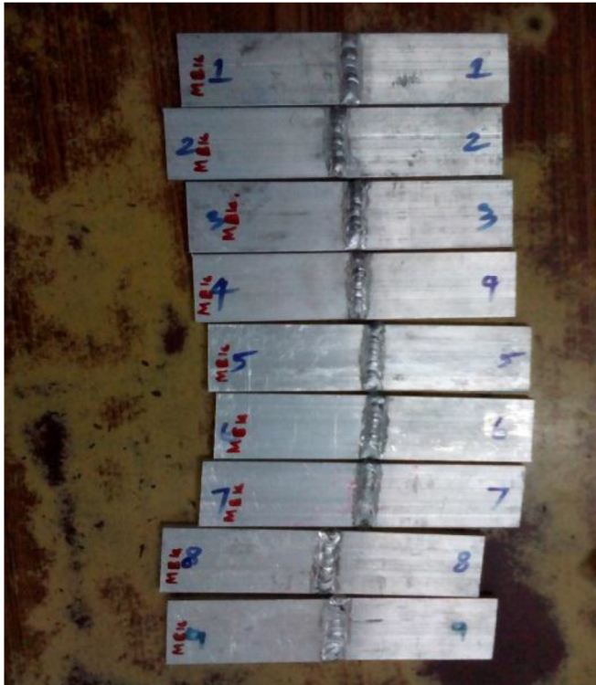
Fig4. Plates after TIG Welding
