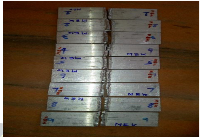
Fig5. Plates After Tensile Testing
