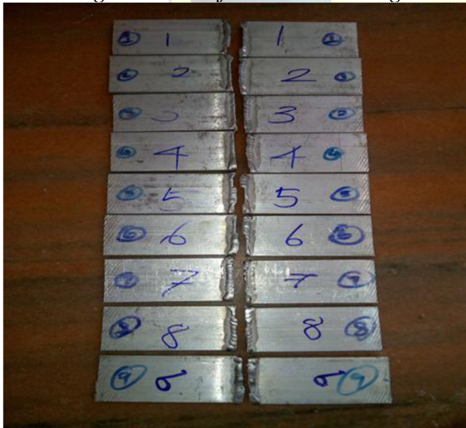
Fig4. Plates after TIG Welding
