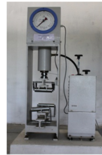
FLEXURAL STRENGTH TESTING MACHINE
