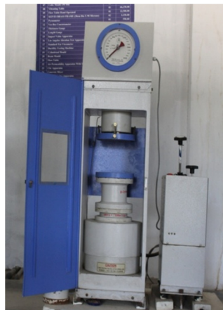
COMPRESSIVE STRENGTH TESTING MACHINE
