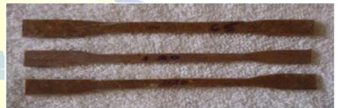
Fig1: Tensile Test Specimen Before Test
