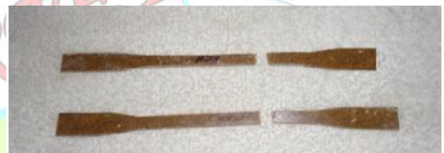
Fig 2: Tensile Test Specimen After Test
