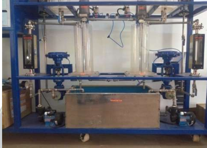
Fig 1: Experimental setup of two tank interacting system
