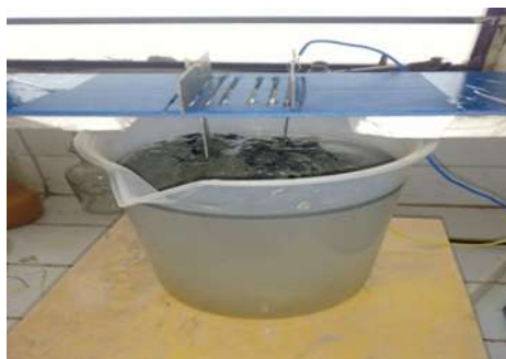
Fig 1: Electrocoagulator and Electrodes used in EC technique
