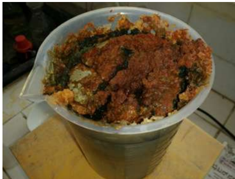
Fig2. Formation of floc during EC process
