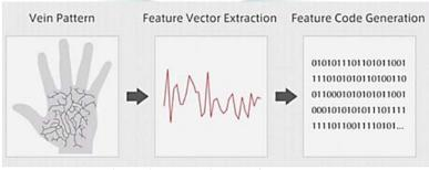
Figure 3: Palm vein scanning process.
