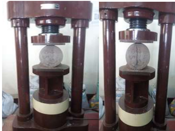
Fig 3. Cylinder Testing Under Compressive Testing Machine
