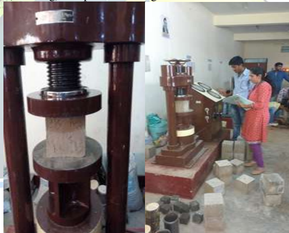
Fig 2. Cubes Testing Under Compressive Testing Machine
