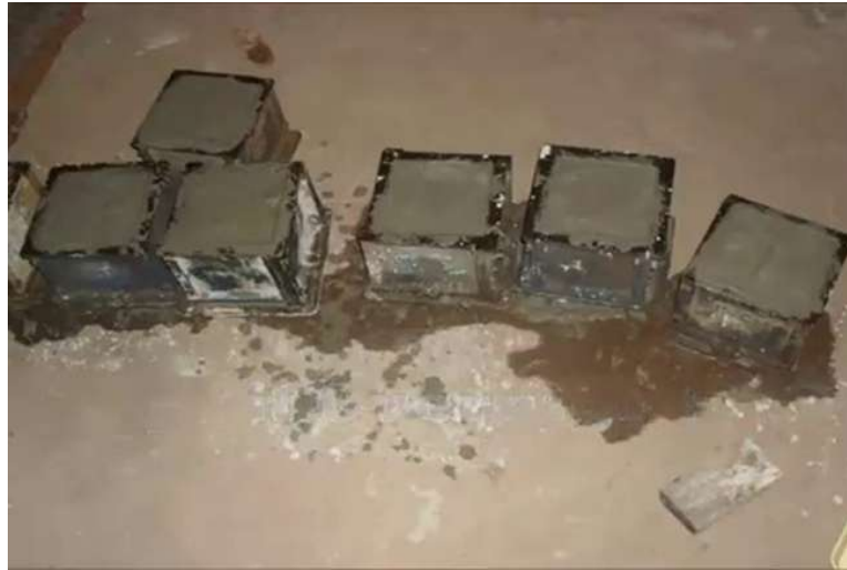
Fig 3: Casting of concrete cubes
