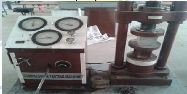
Fig 4: Compressive testing machine
