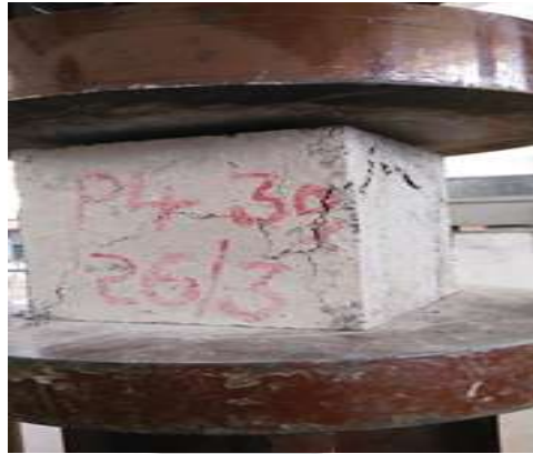
Fig 5. Failure of cubes during compressive test
