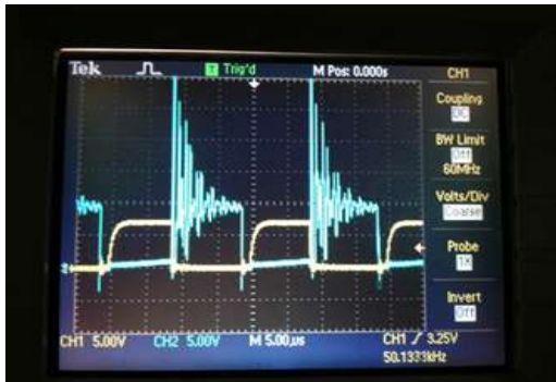
Figure7. Secondary side of transformer waveform
