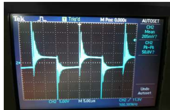
Figure8. VGS and VDS voltage waveform
