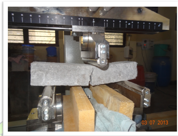
Fig 6: Experimental setup for peak load test
