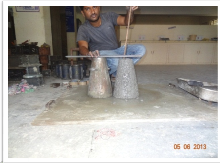
Fig 3: Measuring slump value
