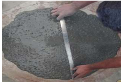
Figure 1: Slump flow test
