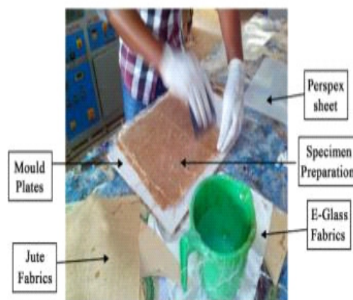
Fig1:Laminates making using hand lay-up technique.
