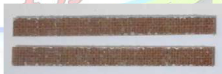
Fig4: Flexural test specimen,
