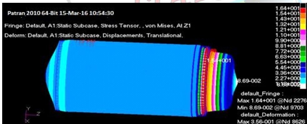
Fig 10: At thickness Z1 shows the static stress for von mises stress tensor and maximum stress location
