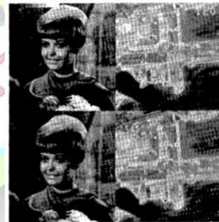
Fig.6 represents the original image (top) and coded image (bottom) of data rate with 2 bits/pixels.
