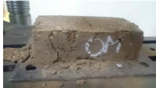
Fig. 6: Failure of unreinforced adobe
