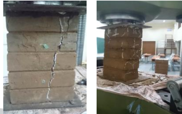
Fig. 9: Crack pattern for unreinforced and reinforced adobe brick masonry
