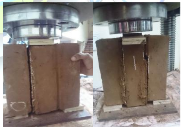
Fig. 10: Crack pattern for unreinforced and reinforced adobe brick masonry triplet
