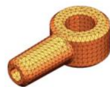
Fig Model subdivided into small pieces (elements)
