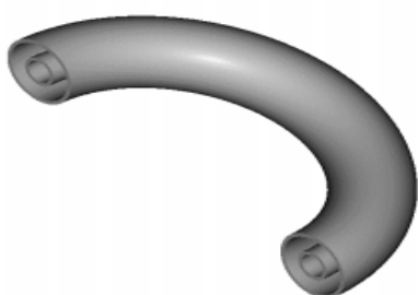
Close-up of double pipe coil
