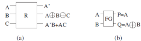
Fig. 4: Block diagram of different Reversible Gates. (a) reversible quantum dot cellular automata (RQCA) gate. (b) Feynman gate
