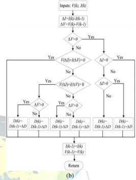
Fig. 2: Inc. Cond. algorithm flowchart (a) conventional (b) Proposed.
