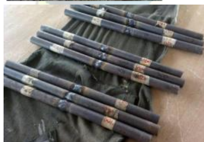
Fig.2. tapered angled and welded mild steel rods
