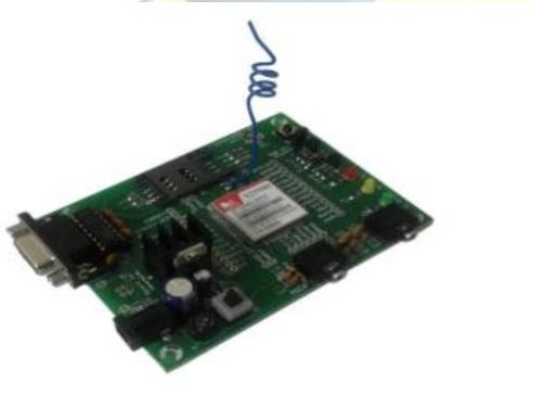
SIM900 GSM module which is extremely popular is used in this project.
