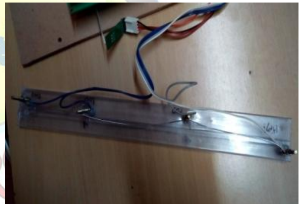
Fig: 5: Capacitive water level sensor
