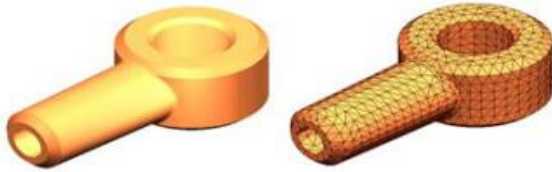
Fig: cad model of a part & model subdivided into small pieces (elements)
