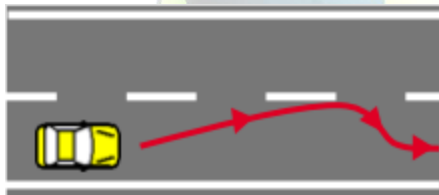
Fig. 1. Lane Monitoring. Show how the vehicle is re-routed on detection of abnormal lateral movements across the lane
