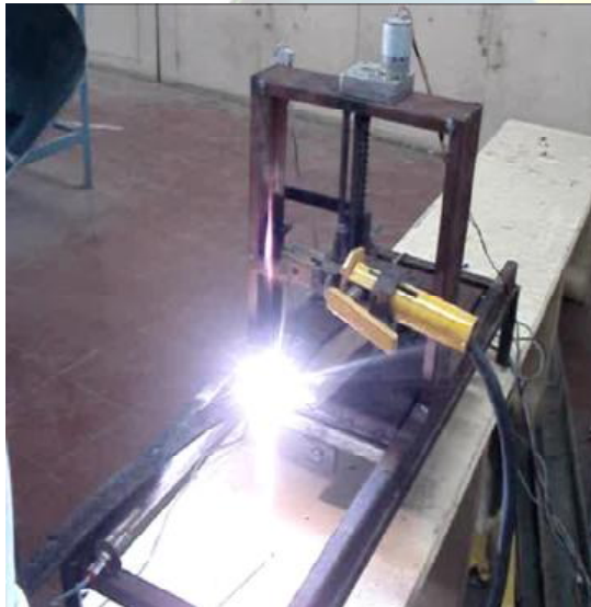
Fig. 9. Working of Slide mode control and automatic electrode feed for arc welding
