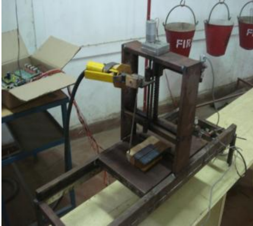
Fig. 8. Slide mode control and automatic electrode feed for arc welding
