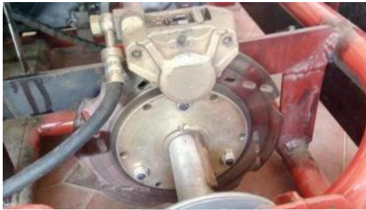
Brake disc mounting
