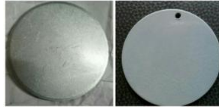
Fig2. Mild Steel disc before coating and after coating
