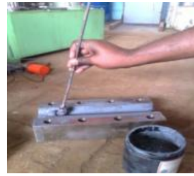
Fig No. 4.1: Coating of die using Wolfrakote TOP
