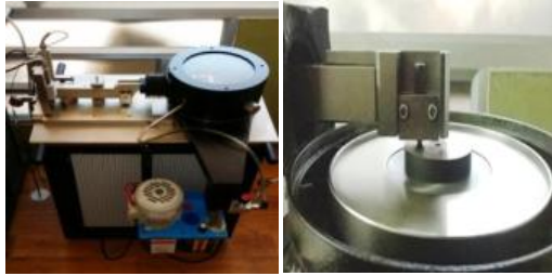
Fig.12 Wear Testing Machine Fig.13 Pin On Disc
